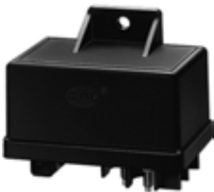
12 V, no. of poles 7, preheating time at +20°C / < 7 sec, Terminal S = postheating cut-out 4RV 008 188-281 Citroën, Fiat, Peugeot
